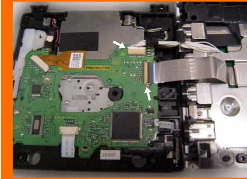
Connect the enclosed flat (short) cable to the latch clip labelled "DVD" in order to connect the Wode interface to the optical drive unit.
