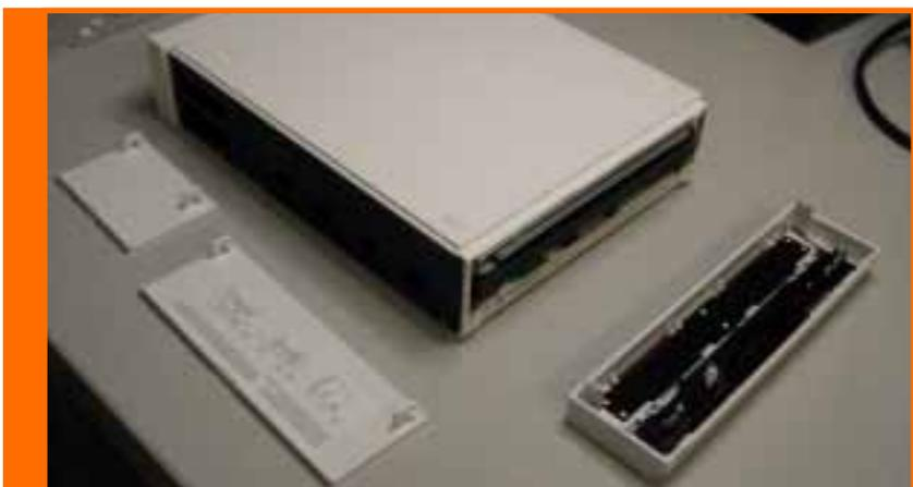
Remove 2 more screws as shown in the picture in order to lift the plastic top cover of the Wii.
