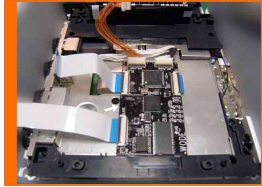
Apply the tape on the top part of the interface in order to avoid possible contacts with the dvd reader.
