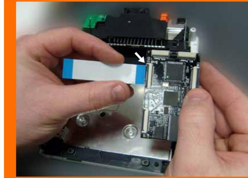
Connect the supply cable (that was connected to the optical drive unit) to the connector labelled "Wii Power".
