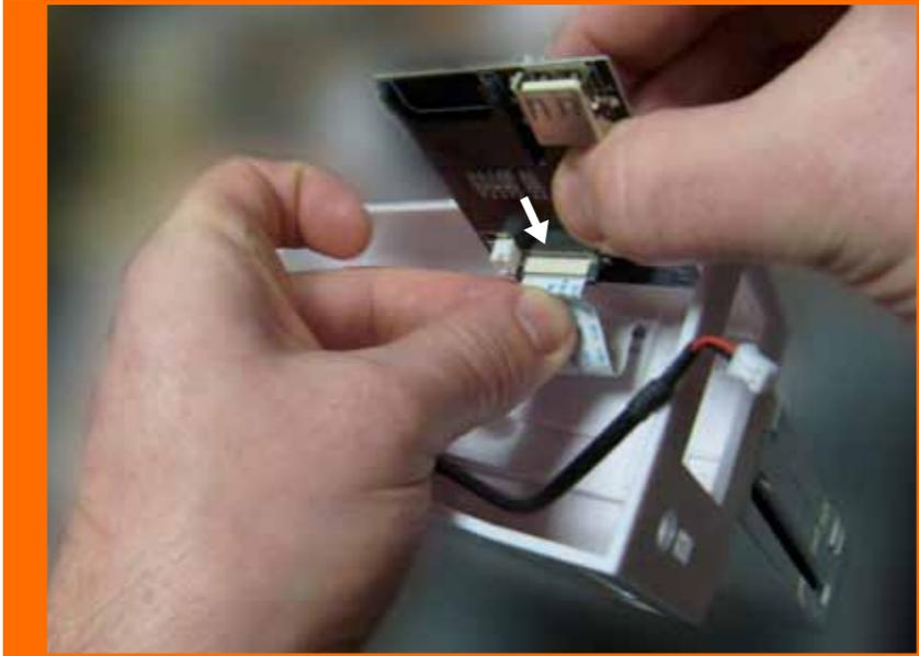
Insert the Slave Board and re-connect the joystick knob.
