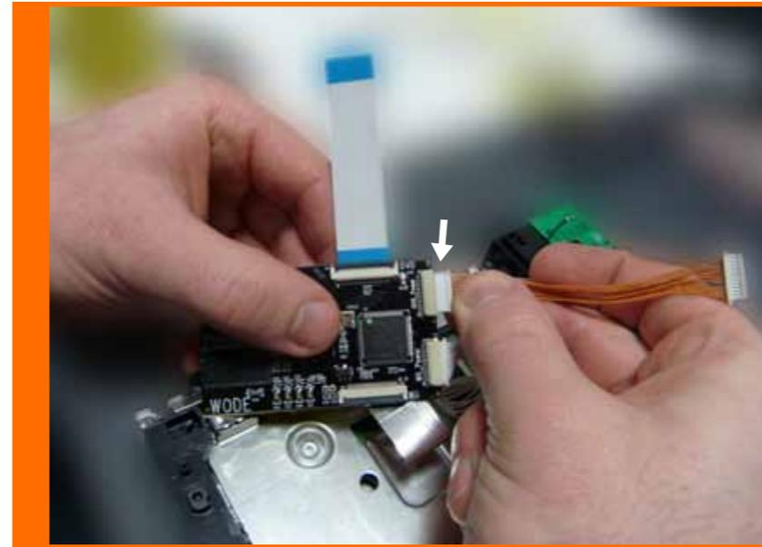
Connect the flat cable from console to the latch clip labelled "Wii" in order to connect the interface to the motherboard of the Wii.
