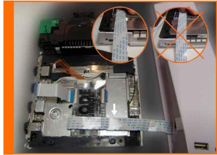
Connect the short flat cable and the supply cable to the optical drive unit.
