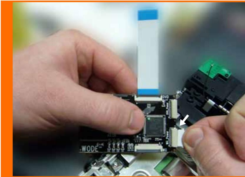
Connect the supply cable from the kit to the connector labelled "DVD Power".
