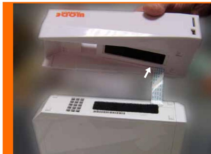
Connect that long flat cable to the Slave Board.
