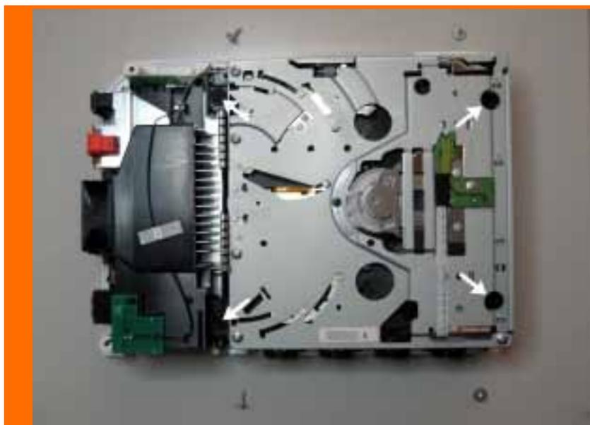
Now lift the optical drive unit so it is off the screw support, and tilt it towards left side in order to put it next to the opened Wii unit. Be careful to not ruin the connector and the cable on the left side that connects the Wii mainboard to the optical drive unit.
