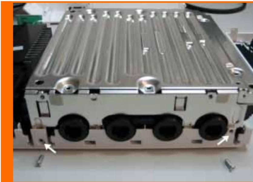
Remove the 4 screws on top of the optical drive unit.
