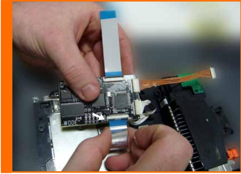
Connect that long flat cable coming from Wode Vertical Stand to the latch clip labelled "SLAVE" in order to connect the interface to the Vertical Tower Display.
