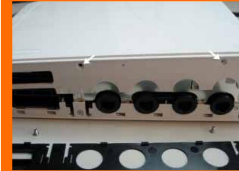
Next remove the 2 tri-wing screws as shown in the picture. This will allow the removal of the metal shield and expose the optical drive unit.
